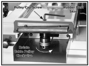
Figure 49. Adjusting cable pulley.
